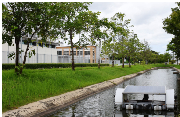
Water turbine powered by solar cell equipped at the Banknote Management Group office
