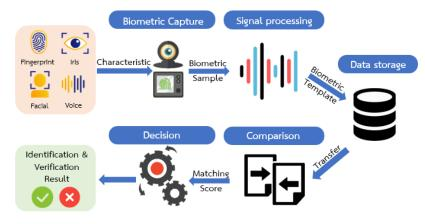
(1) Biometric capture – collects data by using an input device or a sensor that captures the biometric information from a customer and converts it into compatible form for processing. For example, a camera captures a user's face for facial recognition, and a fingerprint reader collects a user's fingerprint.
